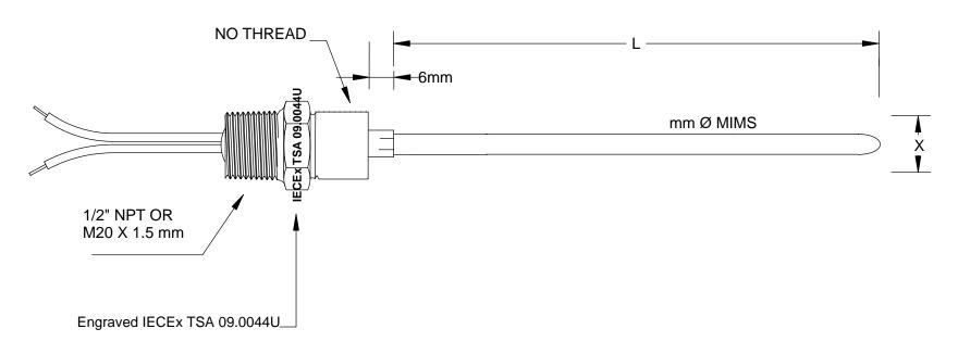
SUITABLE FOR USE WITH CERTIFIED Ex d / Ex e / Ex tD ENCLOSURE OR TRANSMITTER HOUSING WHICH HAS 1/2" NPT OR M20 X 1.5 MM PROCESS CONNECTION
